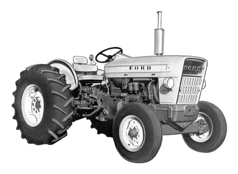
The Ford 4400 tractor delivers ample horsepower for heavy-duty landscaping or mowing with wide flail and rotary mowers. It provides a sturdy power platform for work with 10 or 13-ft Ford backhoes and 3,050-lb Ford loader. A heavy, industrial front axle and support assembly, strong chassis, and sealed, oil-immersed disc brakes make it an excellent logging and pulpwood operations unit.
